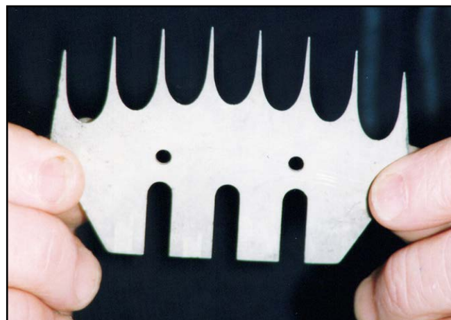
Above: Careful where you go with this beauty – eight teeth, 10cm wide, three comb screws to stop it from warping. A 1970s American item from the Bill Goldsworthy collection.
